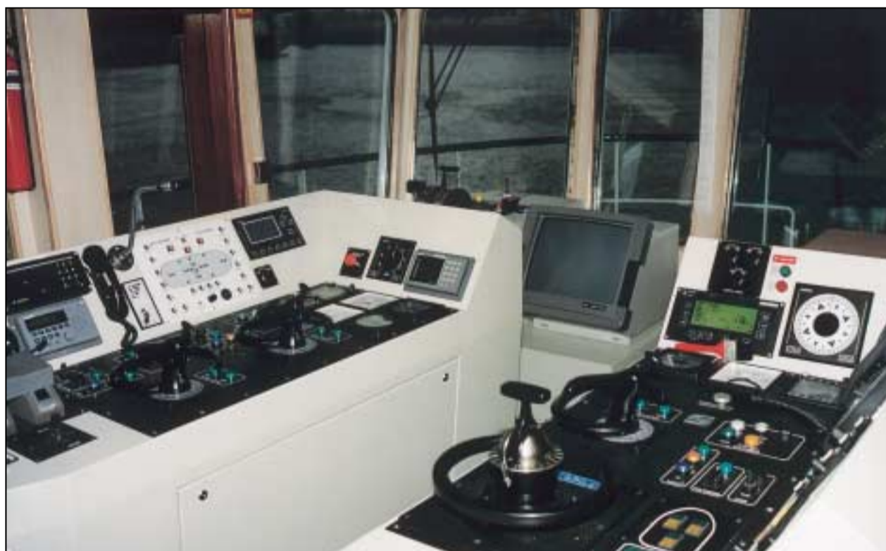
Figure 6 Layout of the bridge, with Master pilot control and independent thruster control handles
